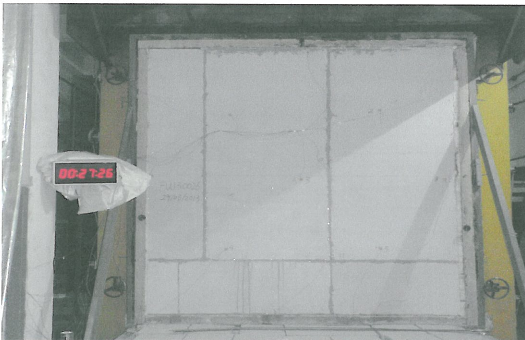
Photo 2 - The unexposed surface of the specimen during the test
