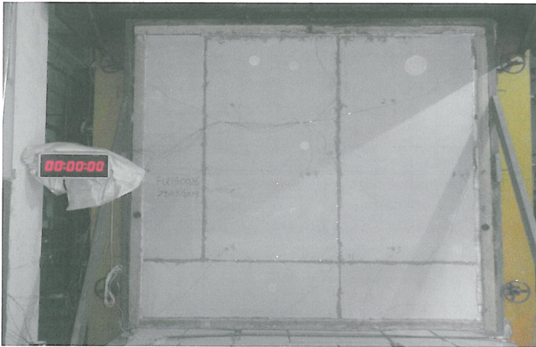
Photo 1 - The unexposed surface of the specimen before the test
