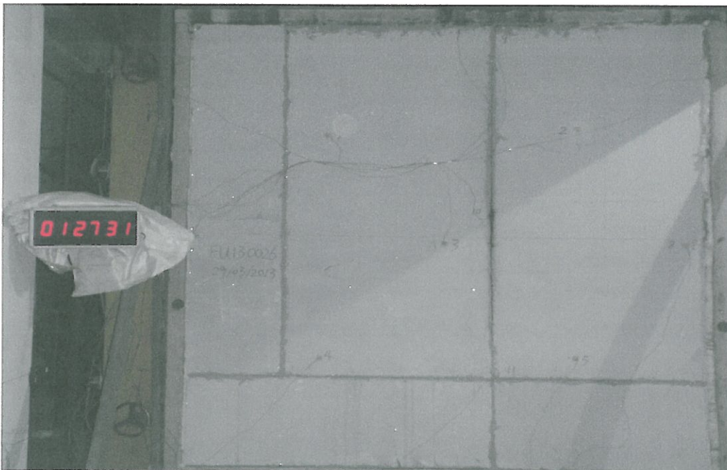
Photo 4 - The unexposed surface of the specimen during the test
